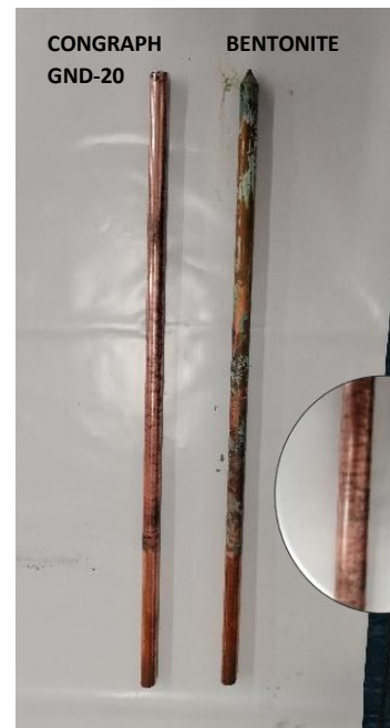
RODS REMOVED AFTER 1 YEAR
